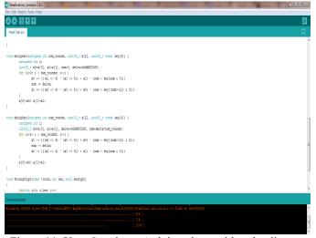
Figure 11: Xtea C code on Arduino along with uploading on Node MCU Esp-8266
