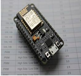
Figure 9: Node MCU Esp-8266
