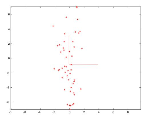
Figure 21.6. A data set which is well represented by a principal component analysis. The axes represent the directions obtained using PCA; the vertical axis is the first principal component, and is the direction in which the variance is highest.
