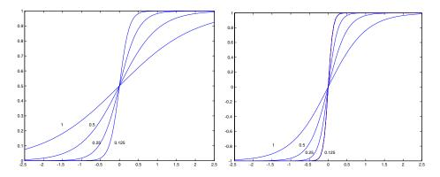
**Figure 21.12.** On the **left**, a series of squashing functions obtained using  $\phi(x;\nu) = \frac{e^{x/\nu}}{1+e^{x/\nu}}$ , for different values of  $\nu$  indicated on the figure. On the **right**, a series of squashing functions obtained using  $\phi(x;\nu, A) = A \tanh(x/\nu)$  for different values of  $\nu$  indicated on the figure. Generally, for x close to the center of the range, the squashing function is linear; for x small or large, it is strongly non-linear.
