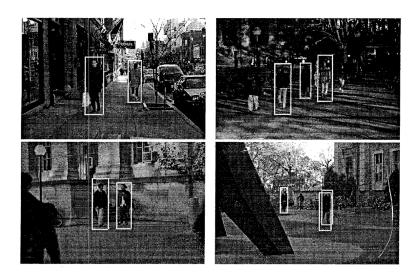
**Figure 21.19.** Examples of pedestrians detected using the method of Papageorgiou, Oren and Poggio. While not all pedestrians are found, there is a fairly high detection rate. The ROC is in figure 21.20. *figure from Papageorgiou, Oren and Poggio, A general framework for object detection, p.3, in the fervent hope of receiving permission*
