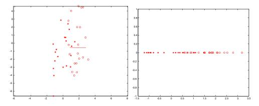
Figure 21.9. Canonical variates use the class of each data item as well as the features in estimating a good set of linear features. In particular, the approach constructs axes that separate different classes as well as possible. The data set used in figure 21.8 is shown on the left, with the axis given by the first canonical variate overlaid. On the **bottom right**, we show the projection onto that axis, where the classes are rather well separated.
