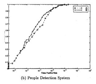
Figure 21.20. The receiver operating curve for the pedestrian detection system of Papageorgiou, Oren and Poggio. figure from Papageorgiou, Oren and Poggio, A general framework for object detection, p.4, in the fervent hope of receiving permission
