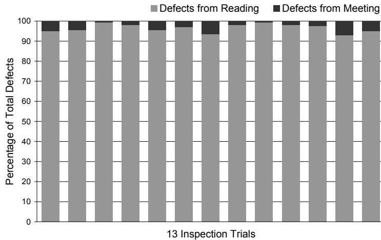
Figure 5: Votta's results demonstrating that inspection meetings contribute only an additional 4% to the number of defects already found by private code-readings.
